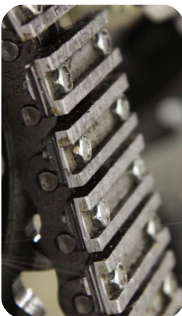
low-cost metal treads designed for ease of manufacture, assembly, and replacement
