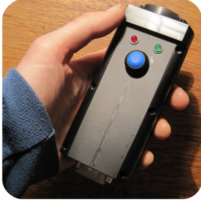
a single thumb-operated button controls the palm-sized timing wand device
