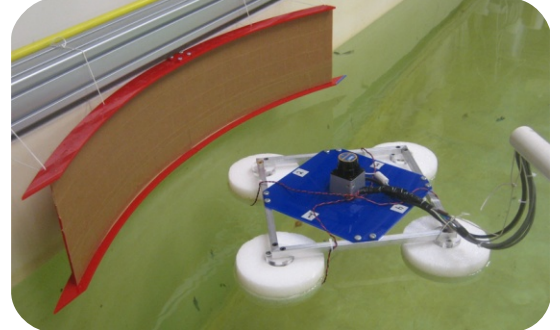
raft robot emulates acoustic sensors for validation of novel control algorithms
