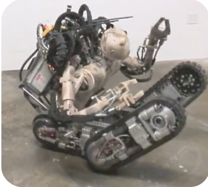
leg segments combine custom rotary hydraulic actuators (hip and knee) with electric-drive tracks
