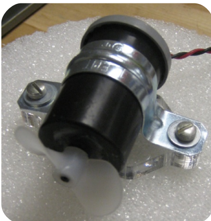
low-cost thrusters constructed from potted dc motors
