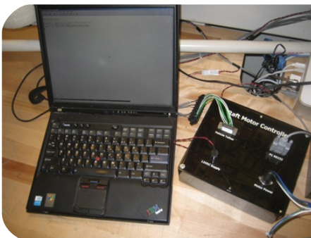
custom microcontroller-based analog motor amplifier and control electronics interface with host pc via an ascii serial interface
