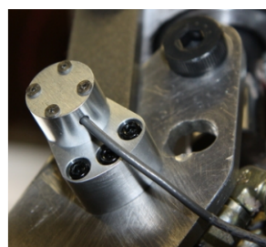
convenient shaft encoder housing packages circuit board for quick integration with general purpose applications
