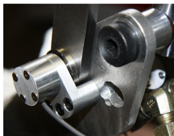
custom encoder mounts and shafting designed to retrofit sensors on bear robot arm joints
